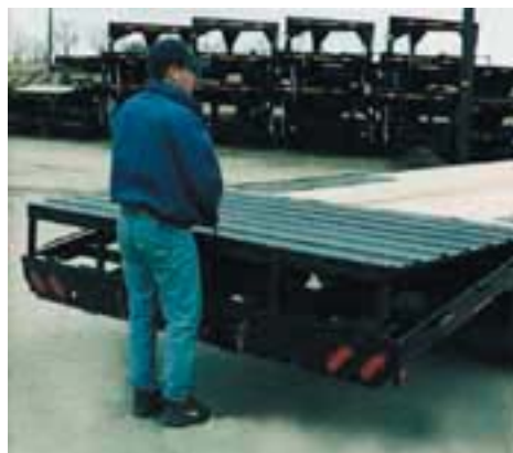
Beaver Tail lifts and locks into place for full length flat bed.
